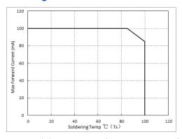
Max Driving Forward Current vs. Soldering Temp
