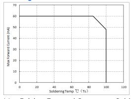
Max Driving Forward Current vs. Soldering Temp
